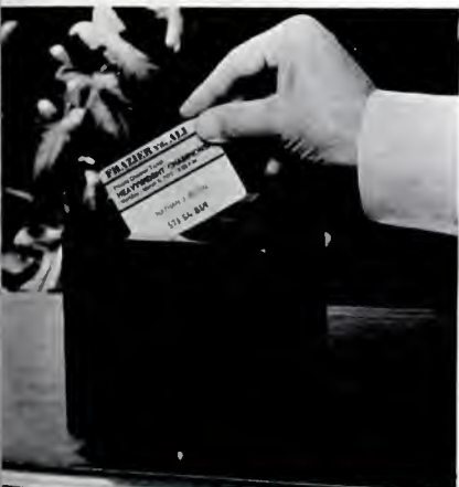
Optical Systems' "black box" uses a plastic card. Pin holes control photocells which activate an unscrambler.
